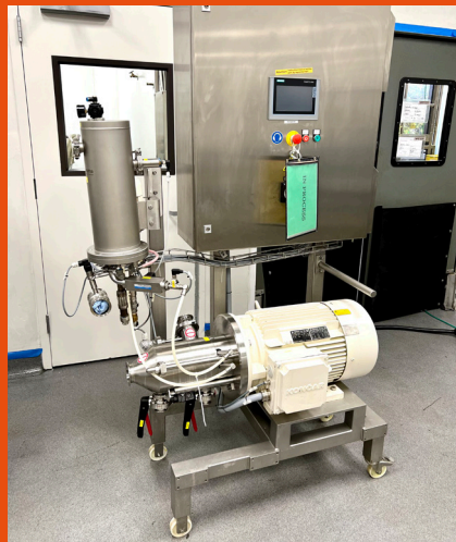
from left to right: installed FrymaKoruma DIL Inline Homogenizer, full view of homogenizer, closeup of CoBall Mill and discharge of the suspension
