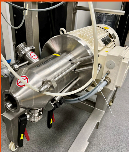
from left to right: installed FrymaKoruma DIL Inline Homogenizer, full view of homogenizer, closeup of CoBall Mill and discharge of the suspension
