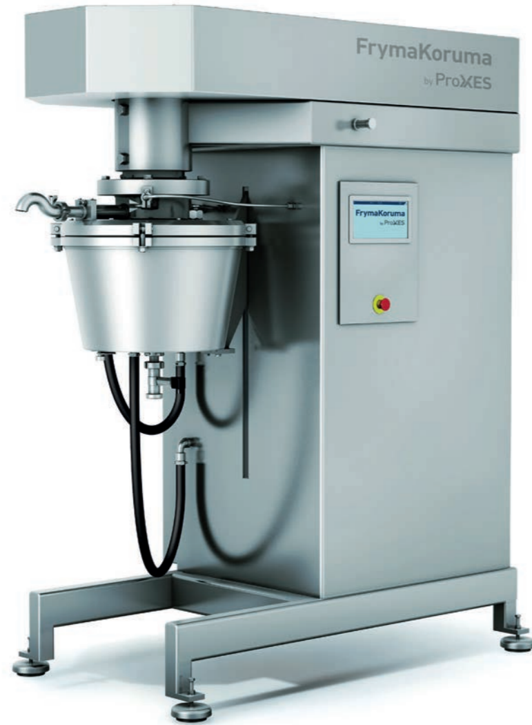
CoBall Mill - MS High energy grinding & dispersing
